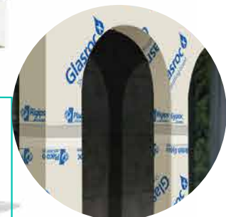
ARCHES Linings to curved surfaces such as arches and columns with minimum bending radius 1,5 m
